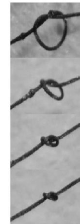
Fig. 14. Micrographs showing the exceptional flexibility of nanotube-based fiber [78].
