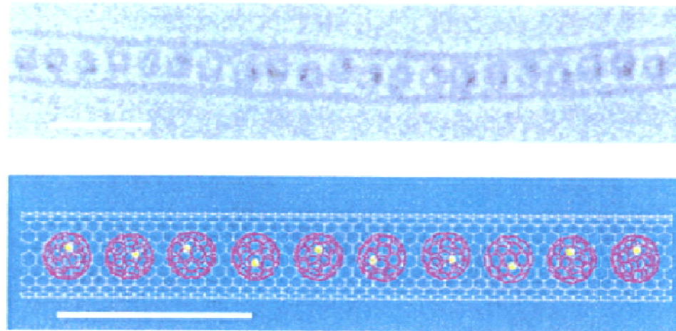
FIGURE 1. A HR image (up) and a schematic model (bottom) of the metallofullerene perope (Gd@C 60 aligned in SWNT) as an example. The dark spots in the HR image correspond to the encapsulated Gd atoms
