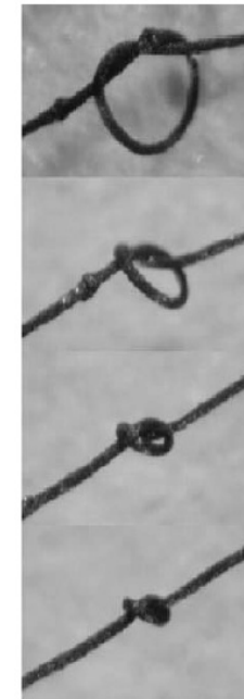
Fig. 14. Micrographs showing the exceptional flexibility of carbon nanotube-based fiber [78].
