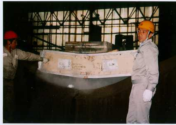
Bending of ice-plugged steel block (10,000 ton press machine)
