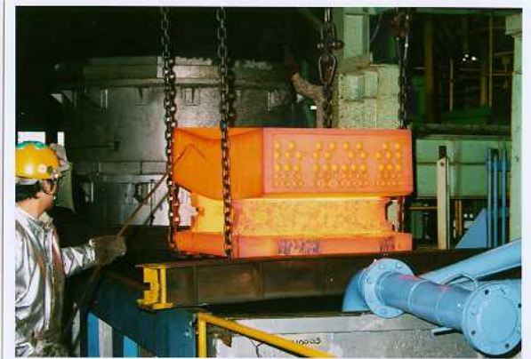
Steel block after solution heat treatment (1010-1054 °C)
