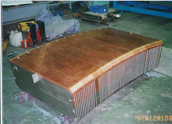
Final assembly of FW and shield block
